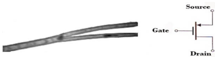
FIG. 3. SEM image (a) and schematic diagram (b) of a transistor built on a Y-shaped carbon nanotube
